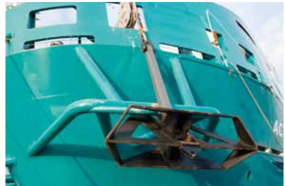
The anchors are connected to steel wires to allow for upgrading to a four point mooring system in the future
