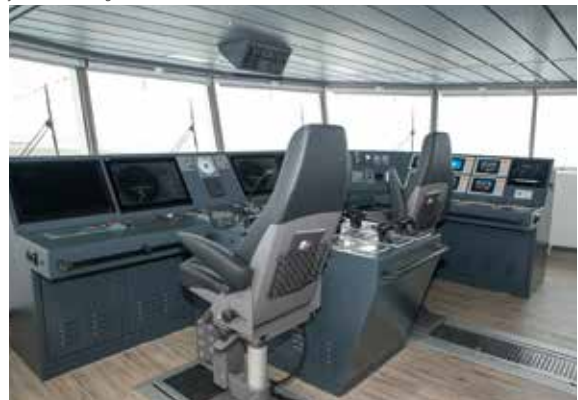
The wheelhouse is separated into two effective bridges: the forward facing part is used solely for transit sailing
