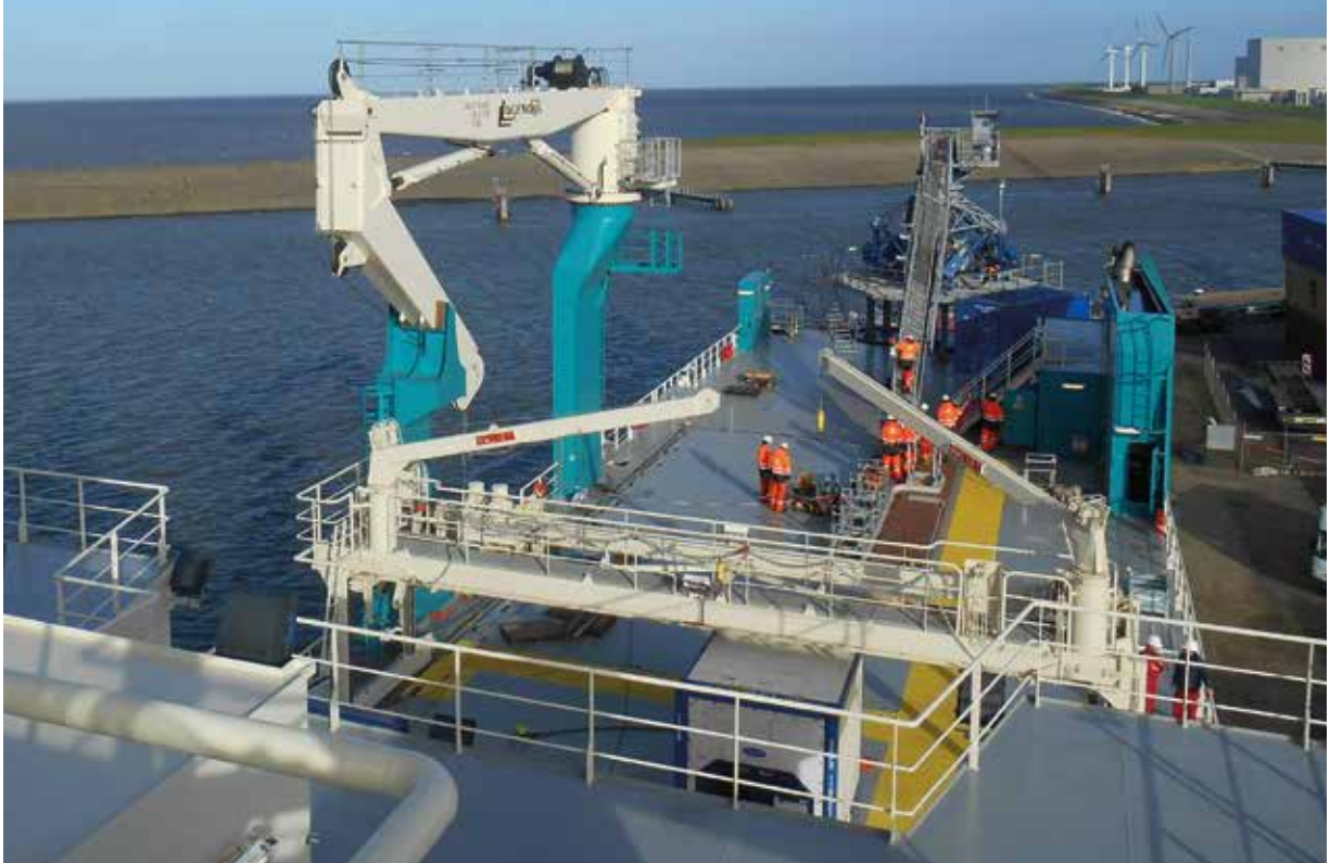
For loading and unloading duties, a semi-custom built knuckleboom crane with a constant tensioning system is provided
