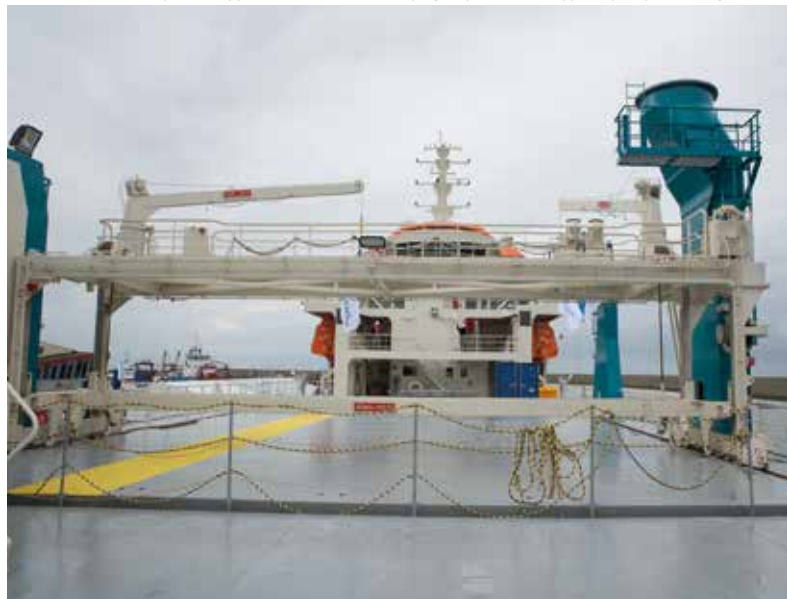
Access to the hold area is provided by four hatch covers, handled by a gantry crane, both supplied by Coops & Nieborg
