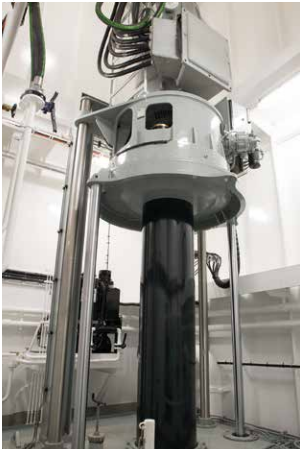
In the bow of two retractable azimuthing thrusters of 750 kW at 900 rpm each, delivered by Veth, are fitted
