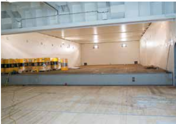
The upper hold acquires its extra length as a result of an enclosed extension over the (lower) engine room
