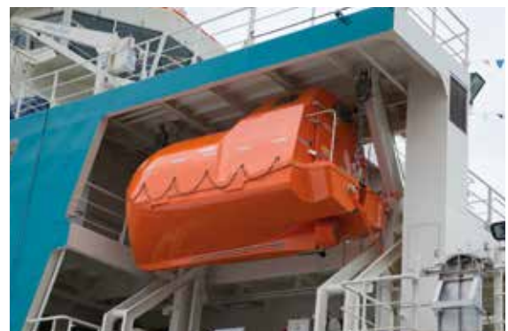
Partially recessed into each aft corner of the superstructure, are the life boats in dedicated davits installations
